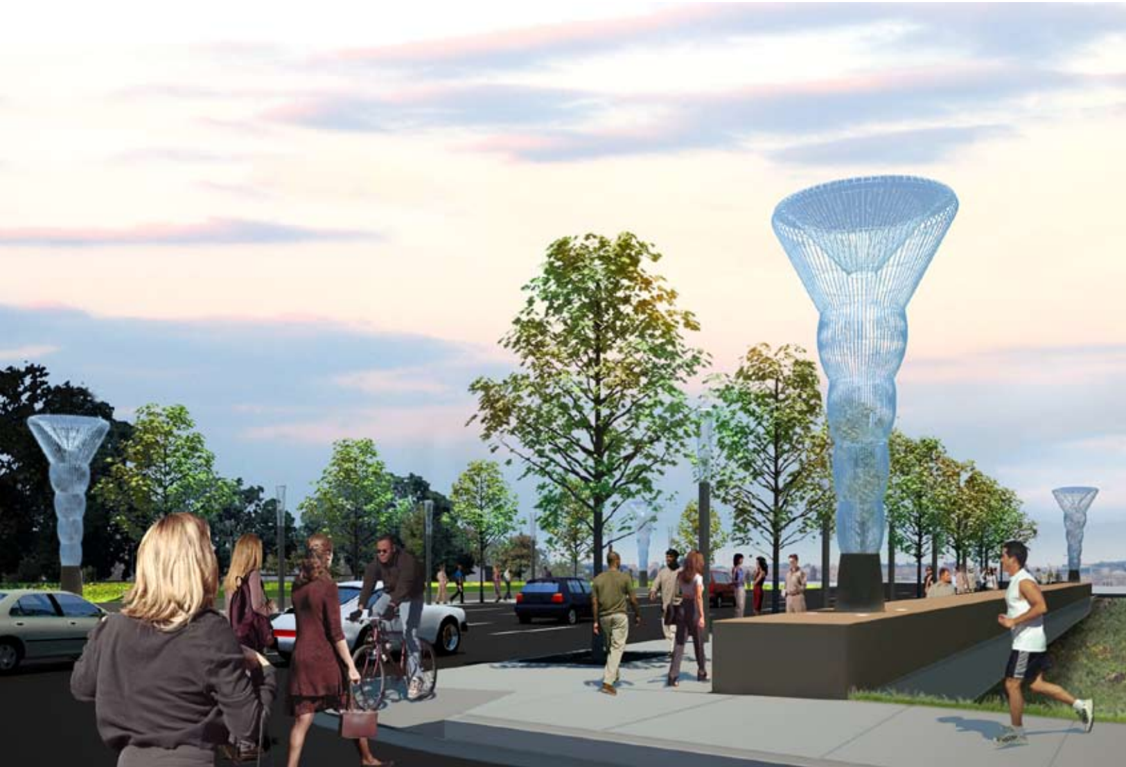
21' Luminous Body (stainless steel, bronze, LED lighting) marking the corners of the Esplanade- looking north 16' Street Lantern (stainless steel, bronze, metal halide lighting) marking the Lynn Street corridor
